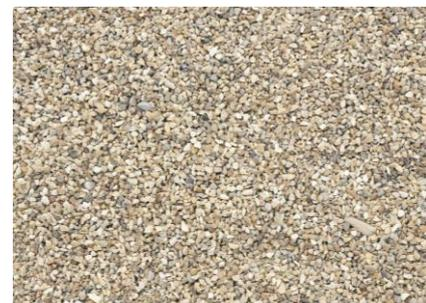
This shows the composition of the dual media filter media used at Orchard Hills Water Filtration. The filter is 2 m deep with a 1.2 m layer of anthracite and 25 cm layer of filter sand grains and a base of larger sand and gravel.
