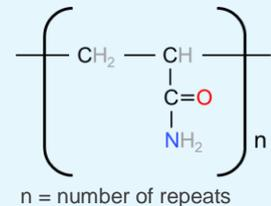
We generally use cationic polyacrylamides that have high numbers of positively charged sites to attract negatively charged organic particles. Anionic polyacrylamide has negatively charged sites used to attract positively charged mineral particles.
