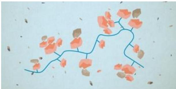
Polymer chain sticking particles together, forming flocs.
