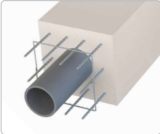
Figure 2 - Reinforced concrete encasement
