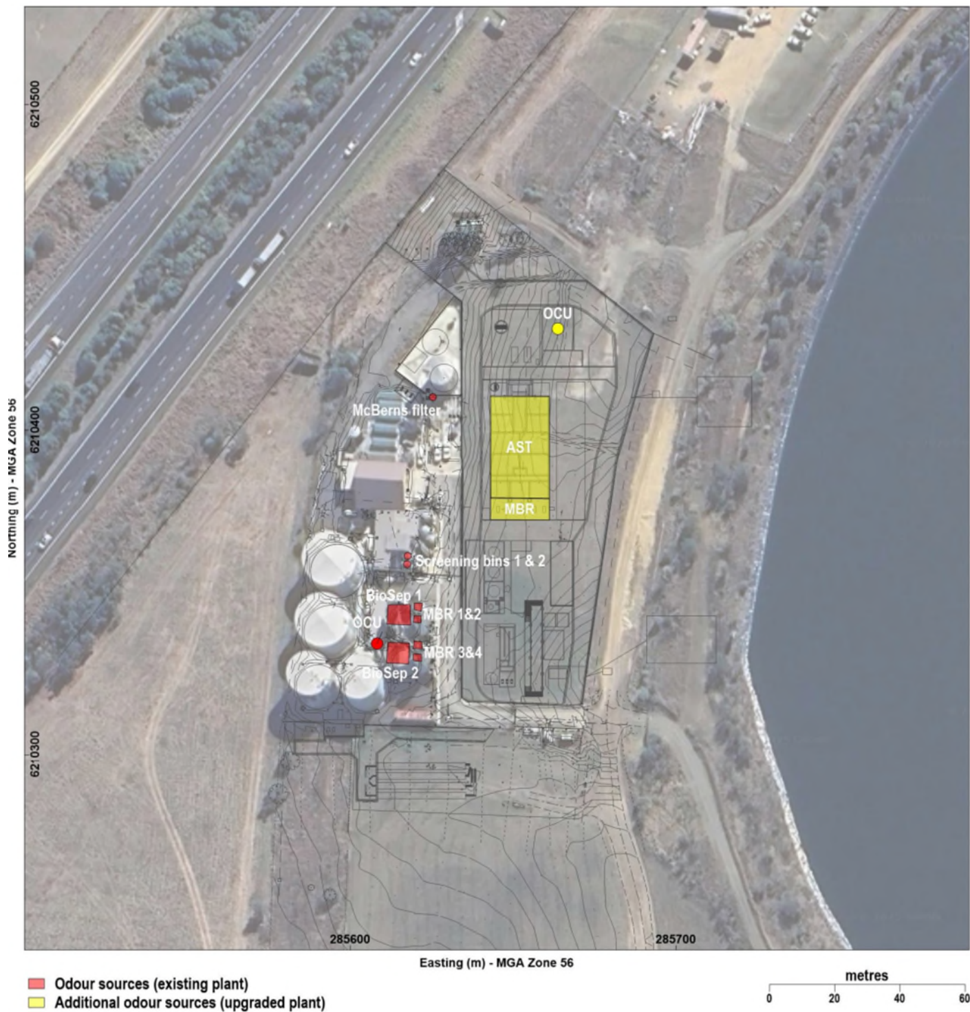
Figure 6-26 Modelled odour sources at the WRRF
