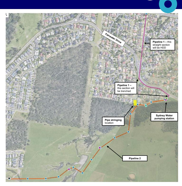
Pipeline 1 will be installed using two construction methods – trenching and horizontal directional drilling (HDD), which means we will a drill the pipe into place underground.
