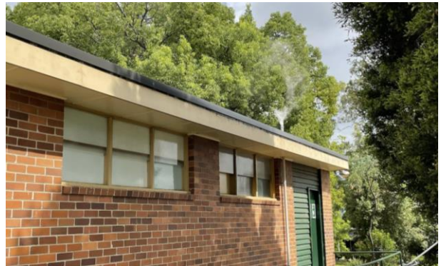
Smoke coming out of a wastewater vent pipe shows that your wastewater system is connected correctly.
