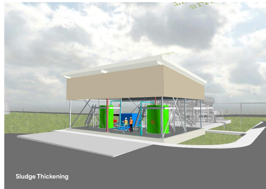
Figure 98 Preliminary design studies for cladding on Sludge Thickening building to reduce solar absorptive criteria.
