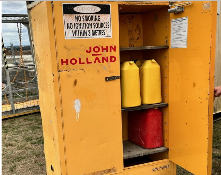
Photo 31: Bunded fuel storage container – AWRC site
