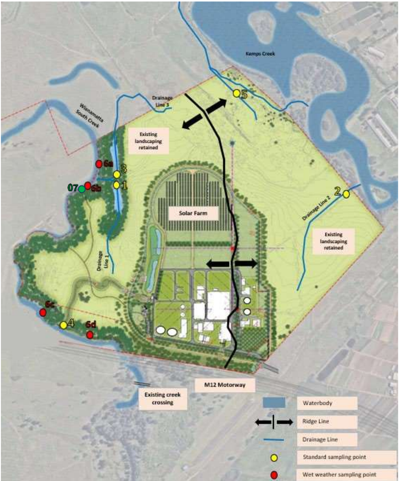
Figure 5.1-1 Surface water construction monitoring locations (AWRC) (indicative only and subject to detailed site conditions)
