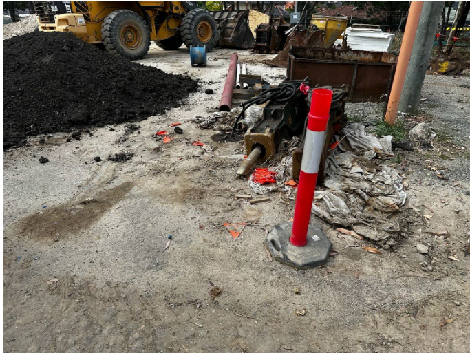
Photo 1: Hydraulic hammer with leaking oil
