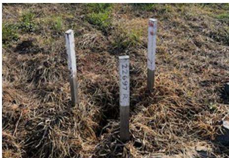
Example survey control mark
