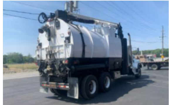
Typical truck used for non-destructive digging
