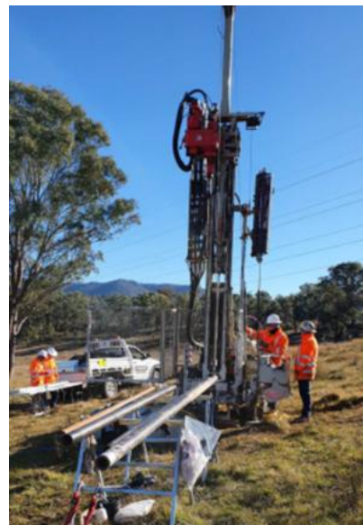
Typical drill rig for drilling boreholes
