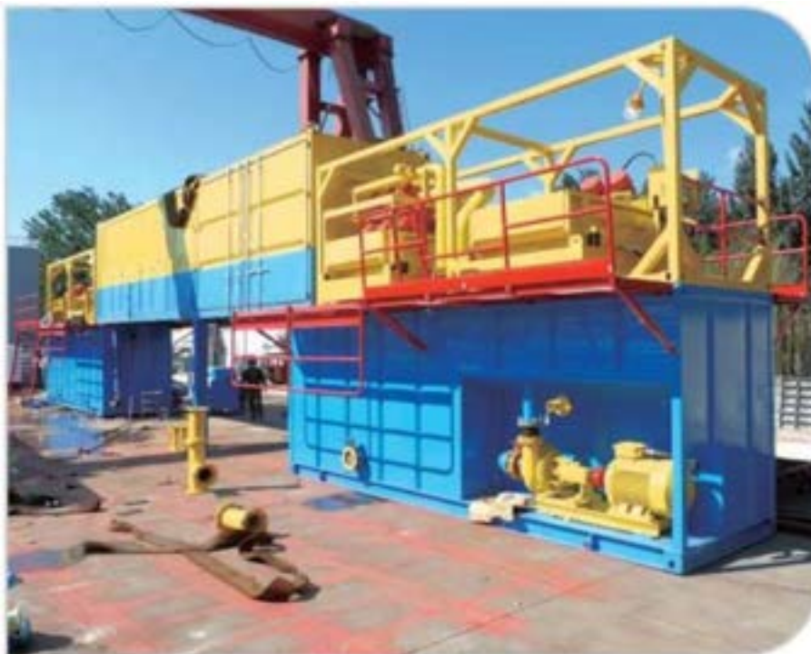
Figure 7: Typical Separate and Bentonite Plan (footprint 3.5m wide x 20m long)
