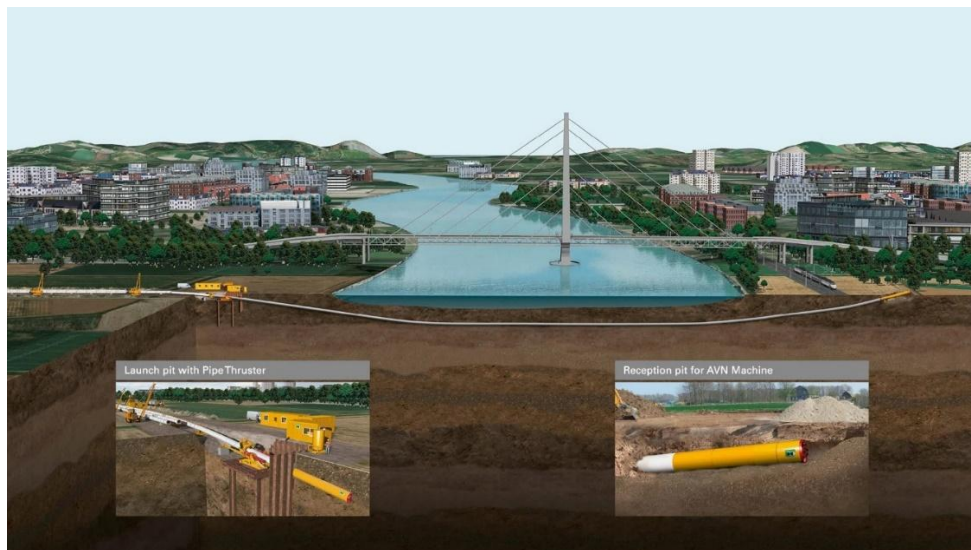
Figure 2-2 Typical direct pipe methodology
