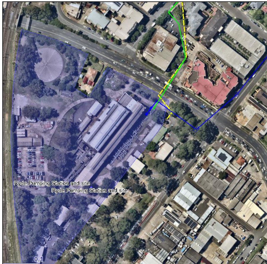
Figure 5-2: Proposed alignment options for the watermain. The green and blue lines show the proposed alignment options. The existing watermain is shown in yellow. Blue shading indicates the SHR curtilage. (Source: Sydney Water)
