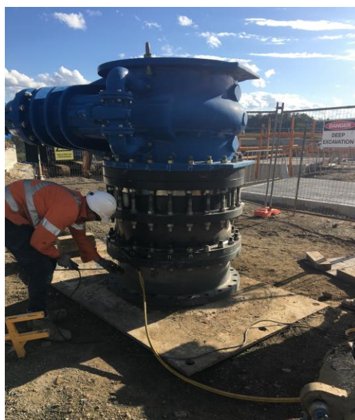
One of the valves undergoing pressure testing.
