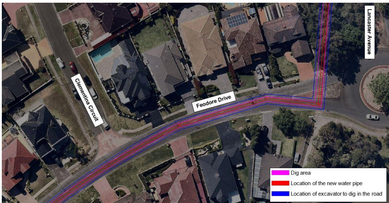
Image showing the extent of the area that will be occupied during installation of the water pipeline along Feodore Drive
