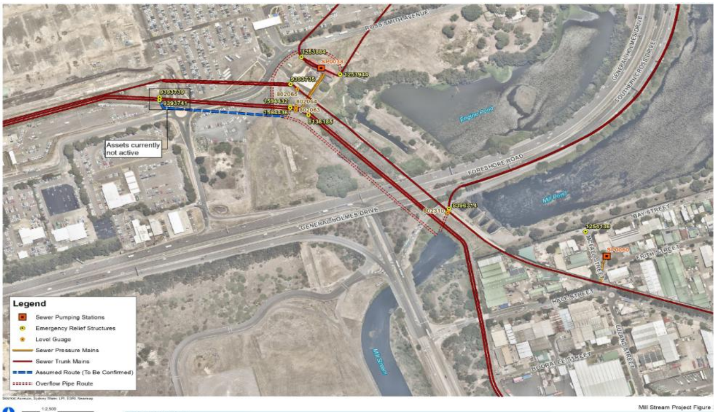
Figure 4 Location of key wastewater assets at Mill Stream, including gauged overflows
