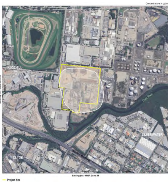
Figure 5-13 Air quality modelling results for PM 10 concentrations
