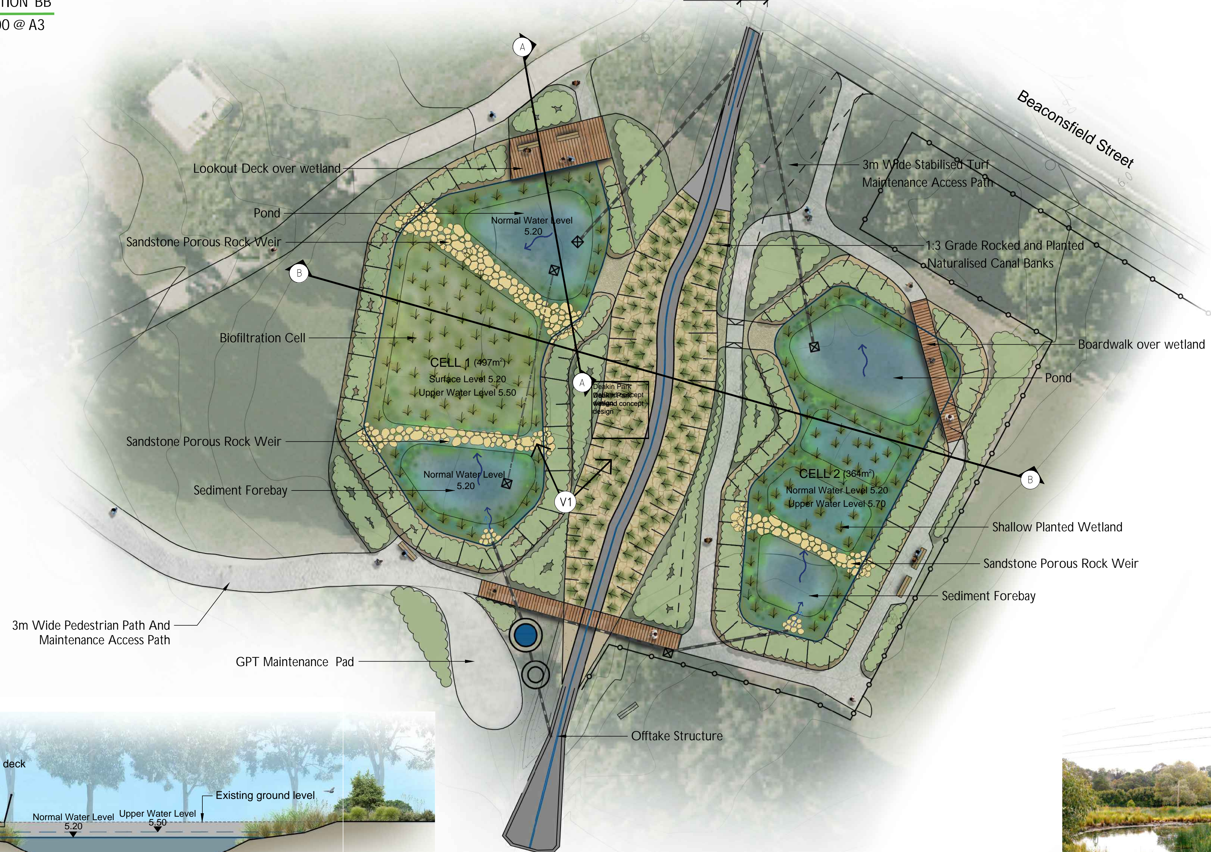
Proposed Naturalised Banks will replace existing concrete/brick channel (Powells Creek)
