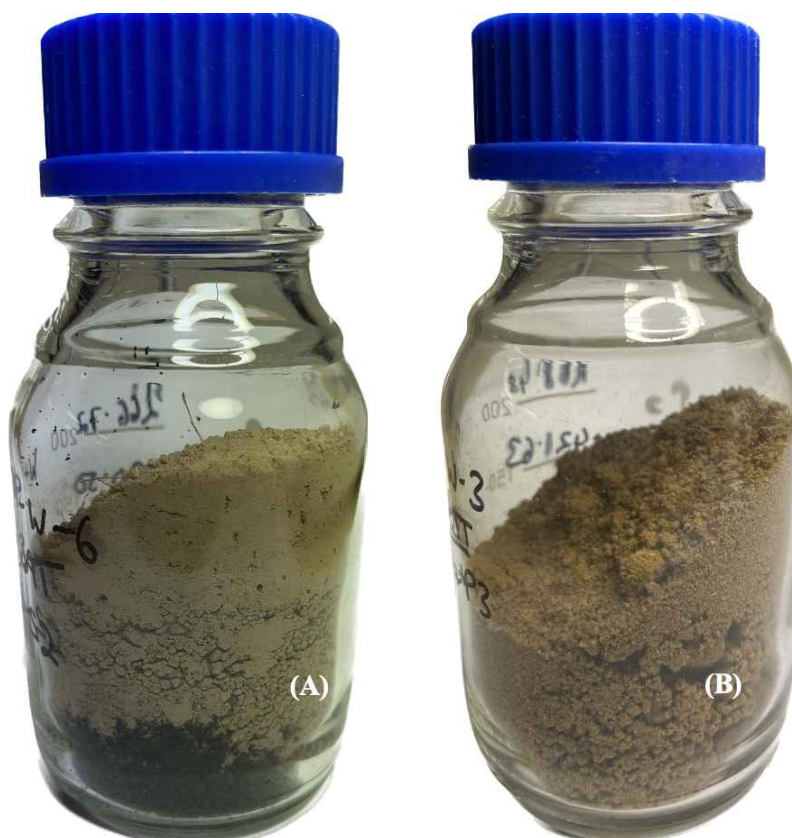
Figure 4 – THB and soil homogenisation (a) Pre-homogenisation with dry soil mass added to THB material. (b) Post-homogenisation step with materials mixed
