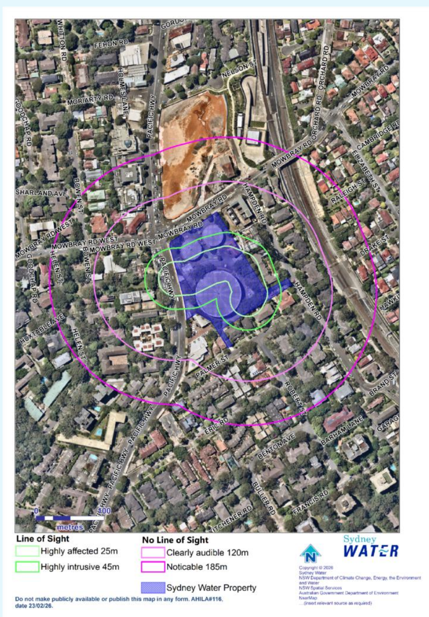
Figure 7 – Affected distance for receivers with and without line of sight during out of hours construction
