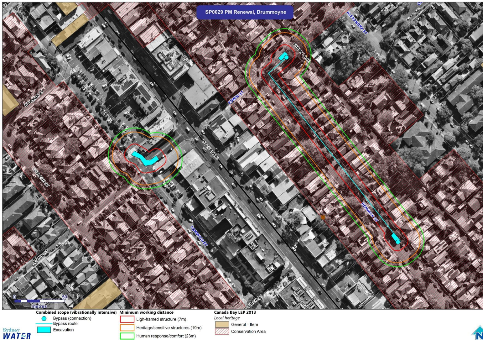
Figure 2-3 Minimum working distances for vibrationally intensive equipment (12-18 t excavator with hammer)
