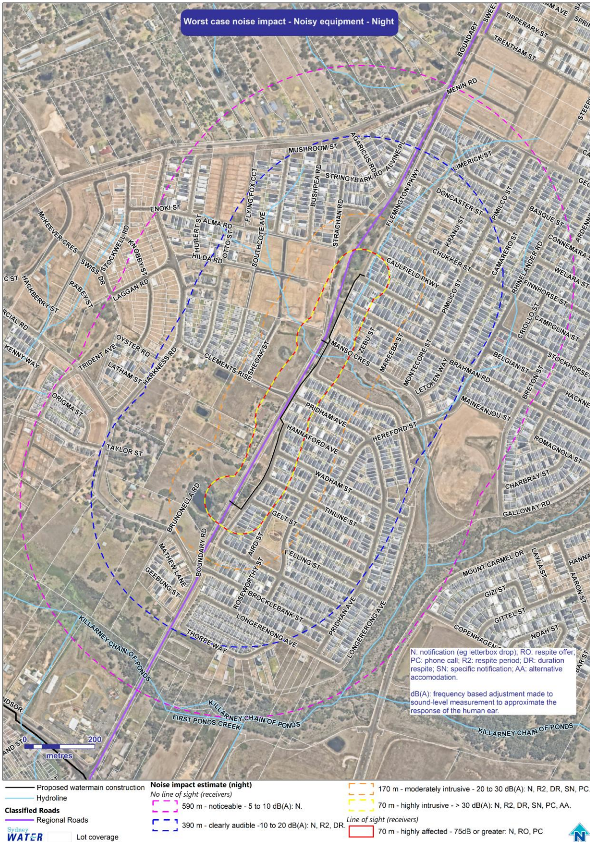
Figure 6 Residential receivers within affected distance during Out of Hours: Night (13.5 T excavator with hammer attachment)
