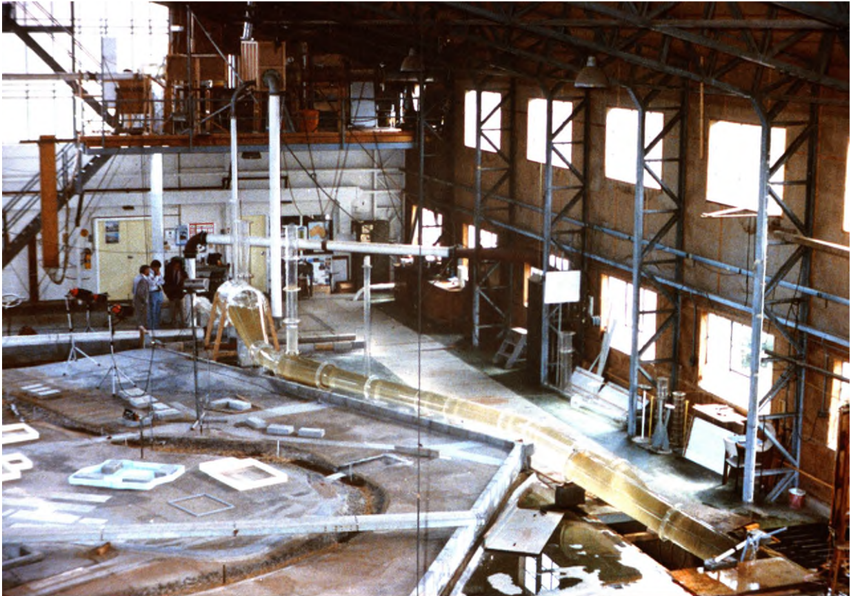
De-aeration Scale Model (1:10) to optimise DOOF design
