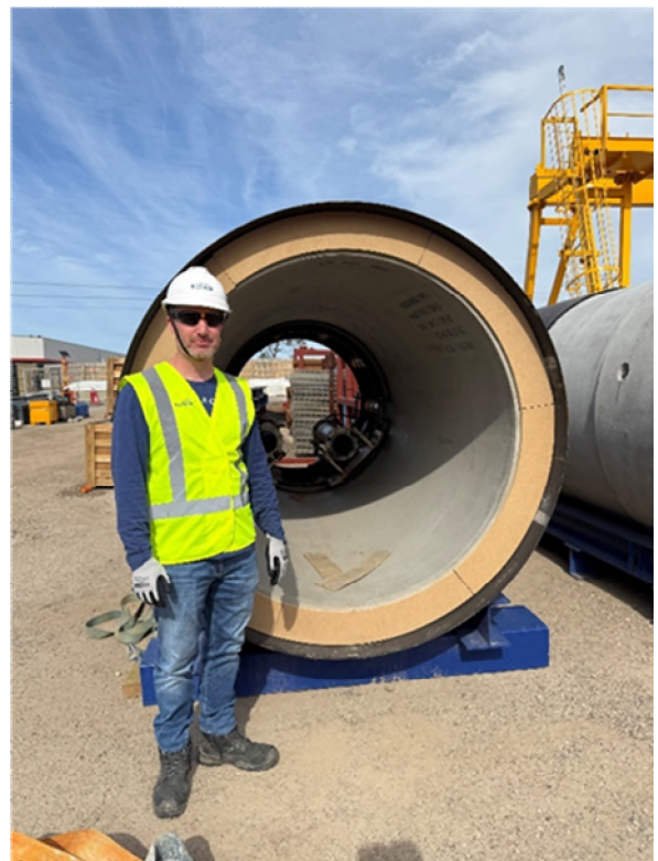
Size comparison of DN1800 Concrete Jacking Pipe
