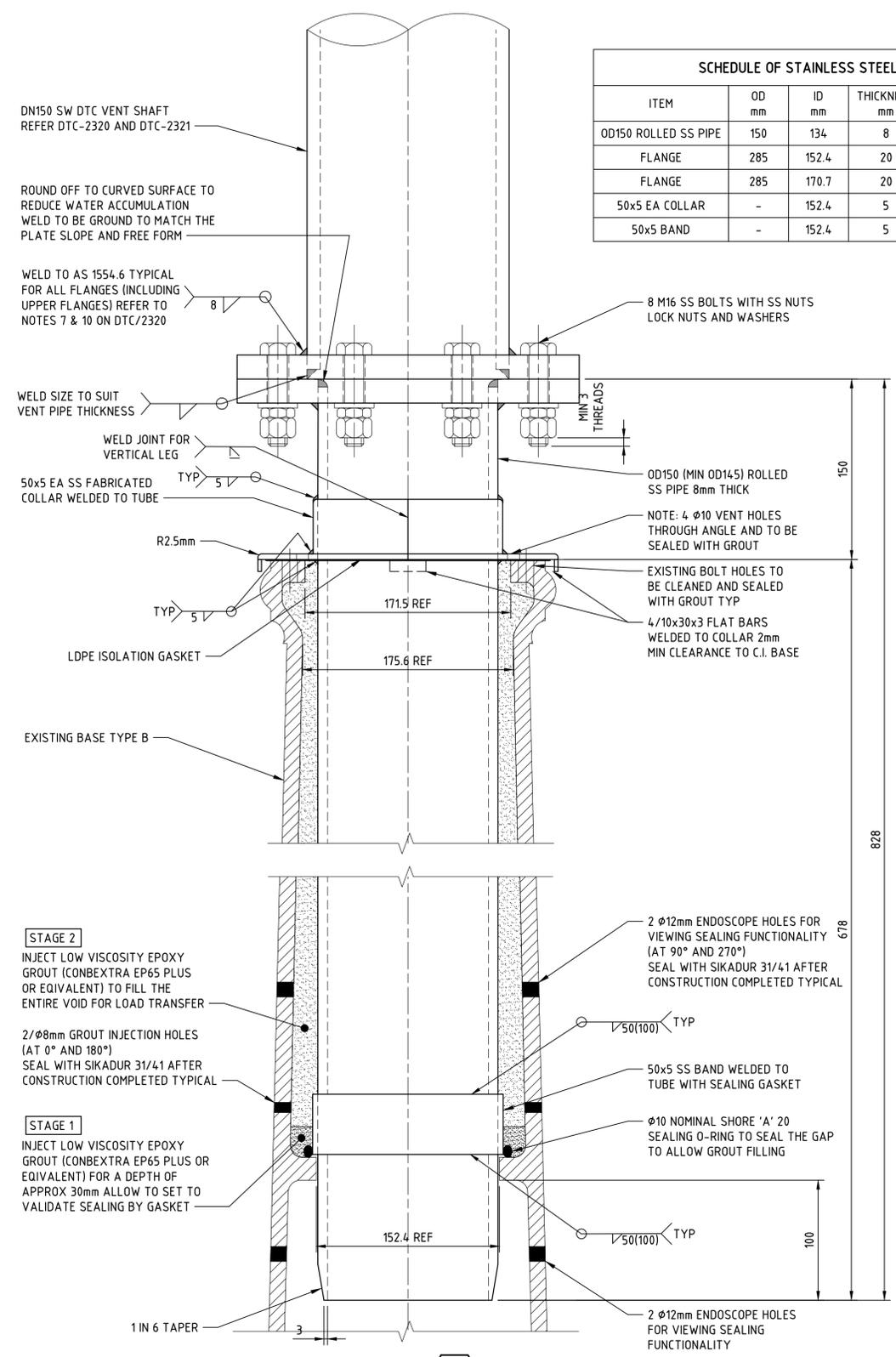
NEW REPLACEMENT VENT PIPE SPOOL PIECE AT TOP SECTION OF STD BASE TYPE B
