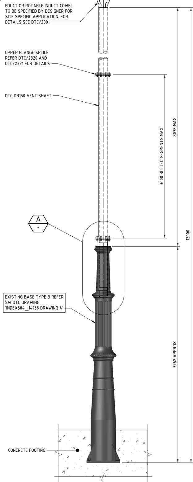
150mm VENT SHAFT WITH STANDARD CI BASE TYPE B
