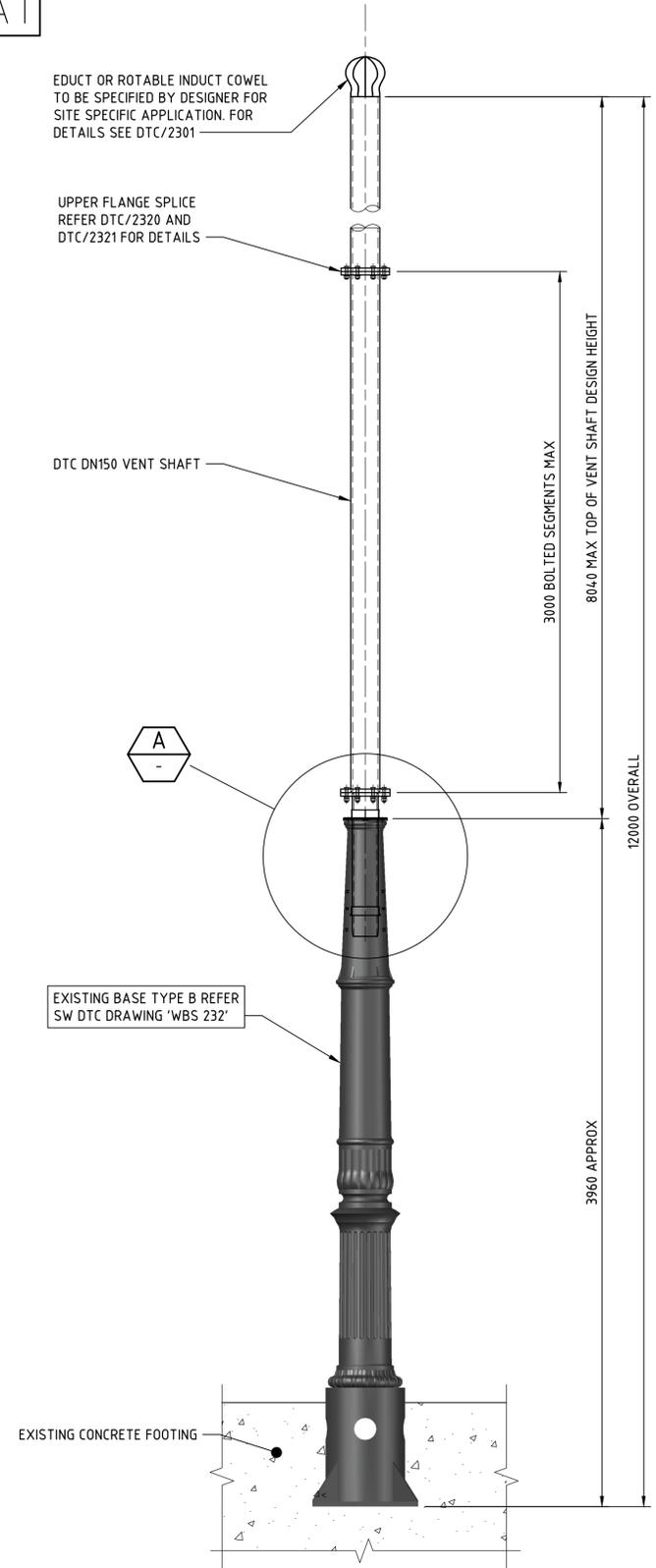
DN150 SWC DTC VENT SHAFT WITH STANDARD C.I. BASE TYPE B
