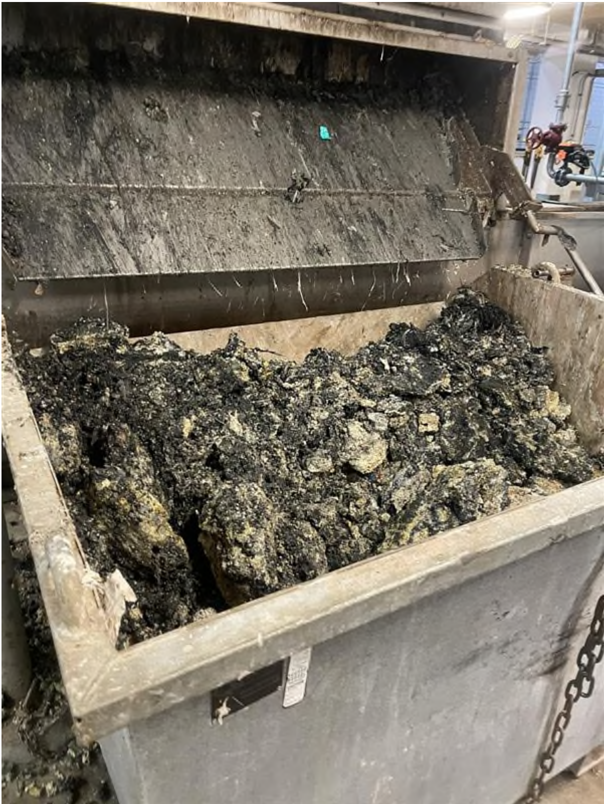
Figure 19: Bin of FOG collected from the Malabar screens during wet weather
