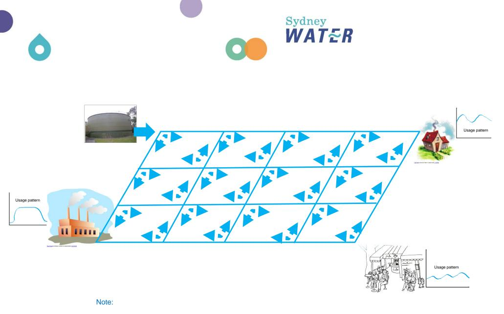
Different land use types (i.e. different peak usage and usage patterns) and different connectivity (e.g. pipe sizes and distance from water source reservoir) lead to constant variation in demand and flow direction during the day with varying demand distribution over time.
