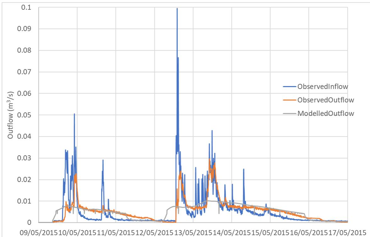
Figure 12 Typical hydrographs for Wicks Reserve following calibration with PEST (May 2015)
