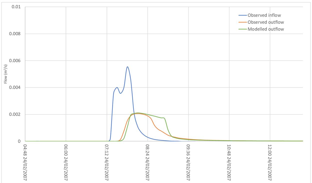
Figure 8 Example events from calibration
