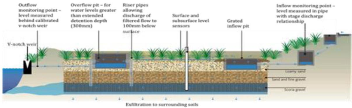
Figure 6-5 Hereford Road biofilter, after (Poelsma et al., 2013)
