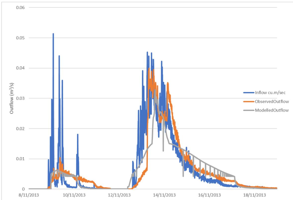
Figure 10 Typical hydrographs for Wicks Reserve following calibration with PEST (Nov 2013)
