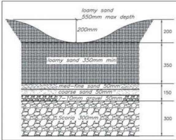
Figure 4 The biofilter cross-section (Bonneau et al., 2020)
