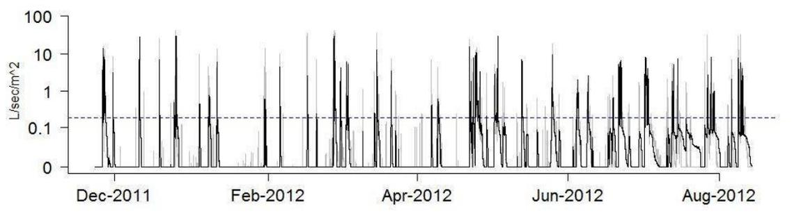
Figure 6-6 Hereford Road long-term hydrograph at outlet (Poelsma, Fletcher and Burns, 2013a)
