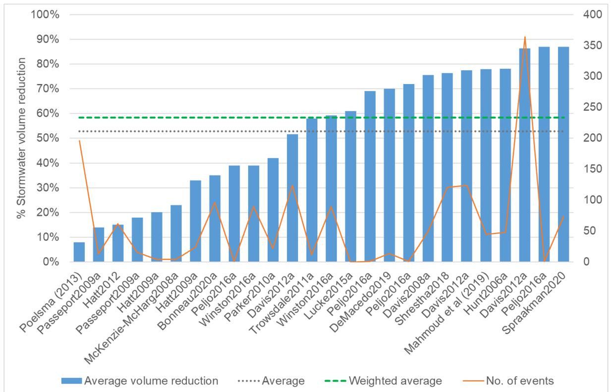
Figure 2 Stormwater volume reductions in bioretention
