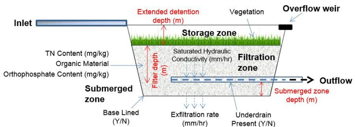
Figure 7 Schematic representation of biofilter in MUSIC indicating parameters of interest (eWater, 2024)
