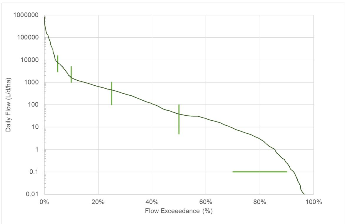
Figure 1 A flow duration curve demonstrating (mostly) compliance with the targets or 'gates'. These are largely achieved by stormwater harvesting but also significantly influenced by outflow rates from assets including bioretention at the lower end of the range
