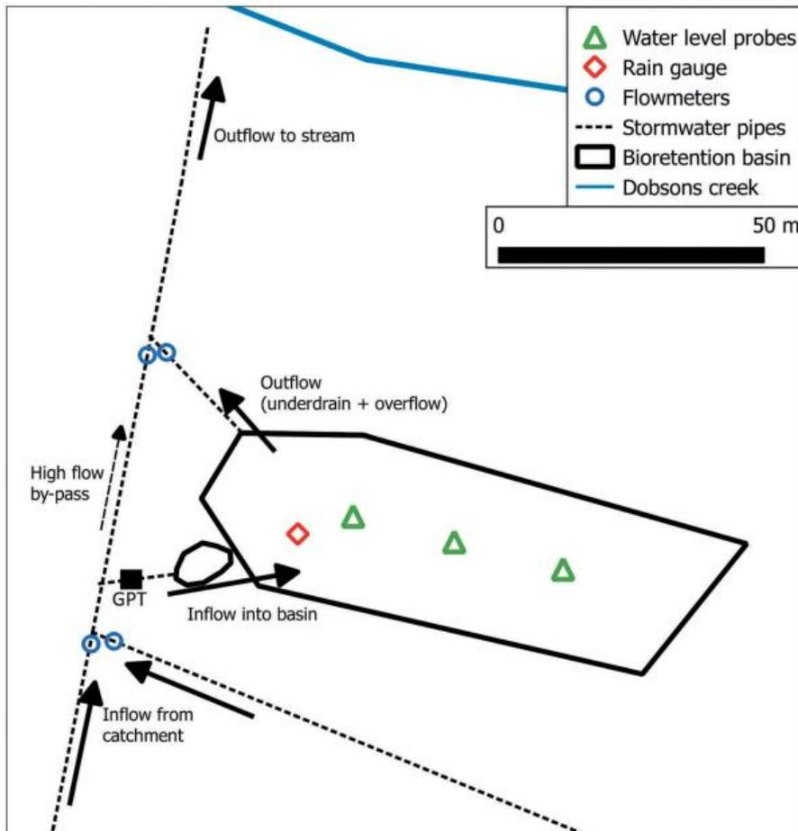
Figure 5 Plan view of the biofilter basin and monitoring systems. Inflows from the catchment are monitored in each of the two inflow pipes, outflows and overflows from the basin are monitored at the outflow pipe and bypass flows are monitored on the high flow bypass.
