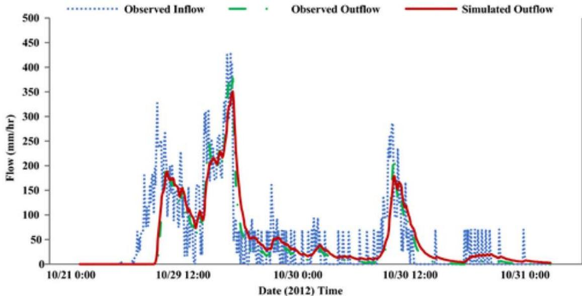
Figure 6 A representative hydrograph for the Villanova BioInfiltration Traffic Island indicating a good fit
