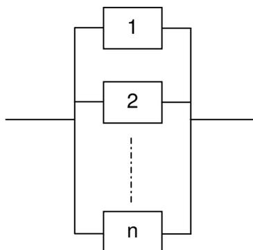
**Figure- 2 Reliability Block Diagram for assets in parallel**
