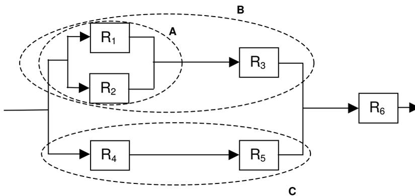
Figure- 3: A system comprised of assets in a combined series and parallel relationship.
