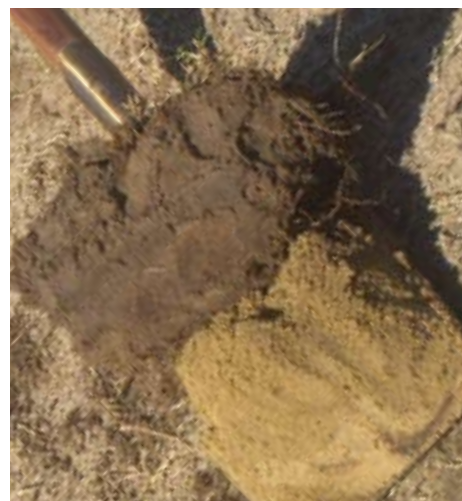
There is a considerable soil depth at this reserve, but the soil is sand that has a low water holding capacity, resulting in very poor turf performance.
