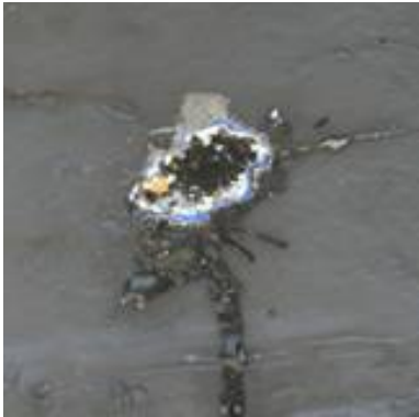
Gelcoat blister with oozing fluid
