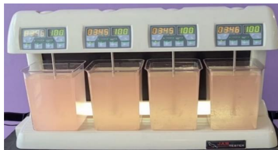
A jar tester is used to model chemical mixing on water treatment plants.
