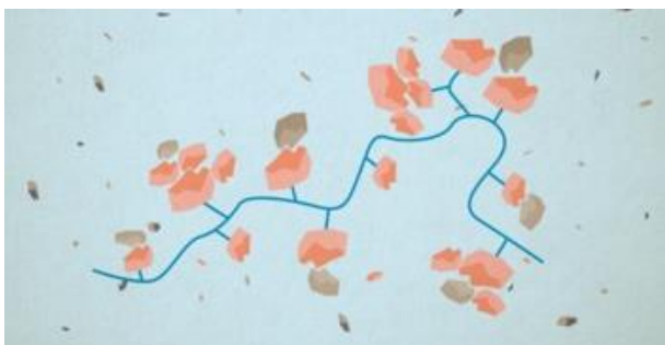
Polymer chain sticking particles together, forming flocs.
