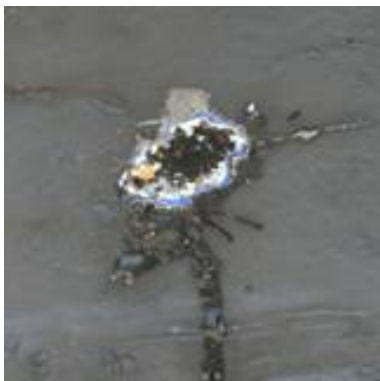
Gelcoat blister with oozing fluid
