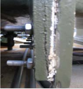
Delamination of a pultruded I-beam flange
