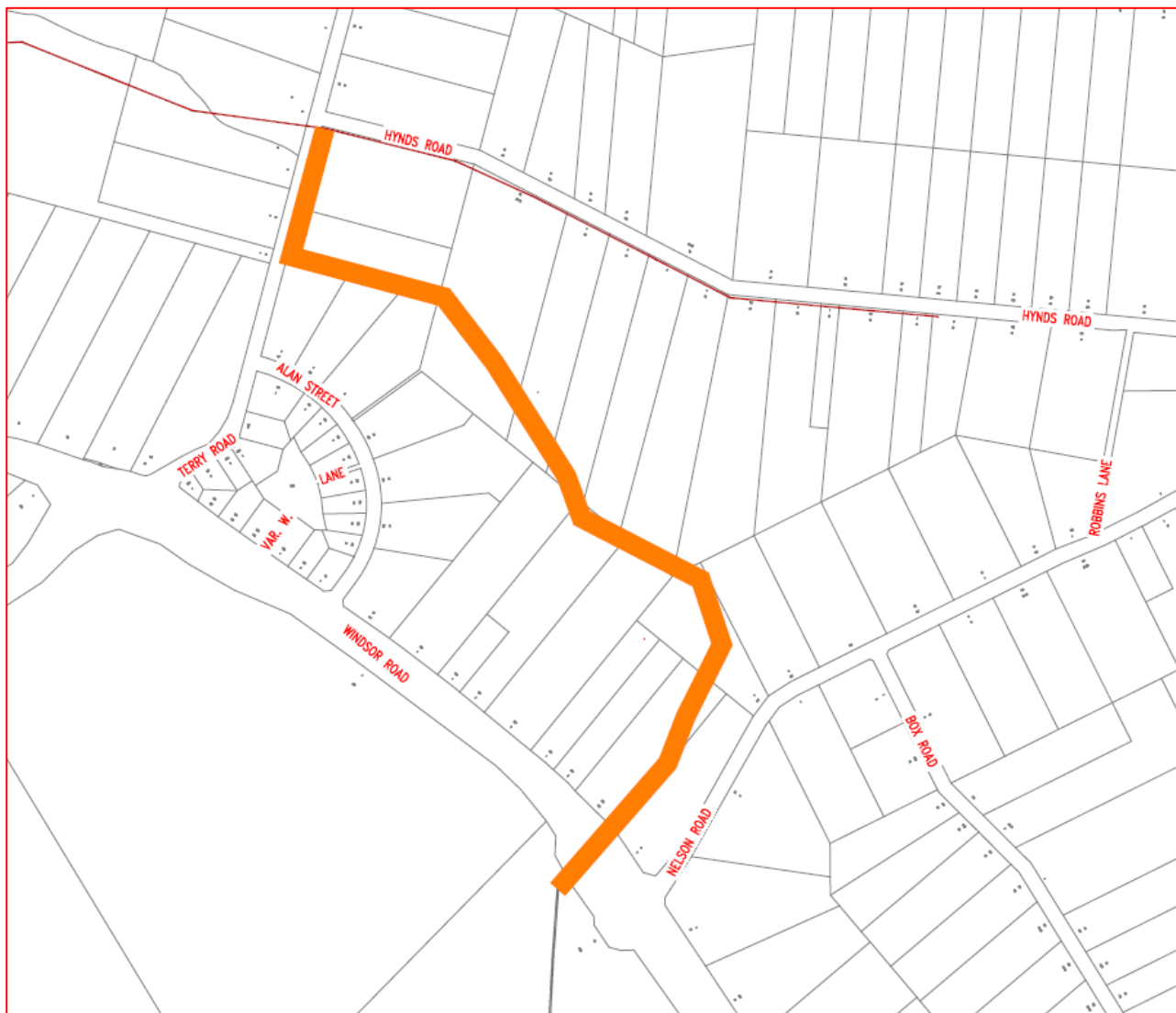
Figure 4 – Approximate location of new wastewater mains near Hynds Road, Terry Road, Alan Street, Nelson Road and Windsor Road, Box Hill
